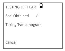
Once an adequate seal is detected the tympanogram measurement is made. This takes about 3 seconds. It is important not to move the probe and to ask the patient to remain very still during the test.
