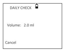
Remove the probe and repeat the test with the three remaining test cavities. The display should show the volume of the 0.2ml and 0.5ml test cavities to within  $\pm$  0.1ml. The 5.0ml test cavity should be within  $\pm$  0.25ml.
