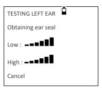
The number of bars shown indicates the robustness of the seal. The probe should be adjusted in the ear until two or more bars are shown for Low & High.
