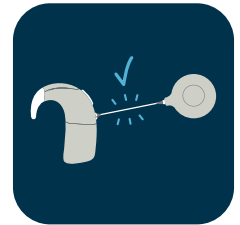
Antenna cable pull – 35 N (3.5 kg)
